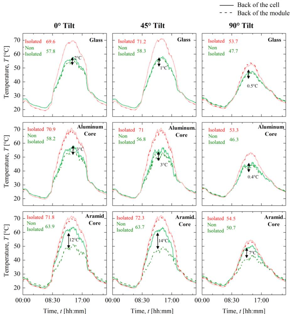
**Figure 5:** Temperature monitoring of the different installations ( $0^\circ/45^\circ/90^\circ$ ) for a typical end-of-summer cloudless day. The cell temperature is represented in red and the back-of-module temperature in green.  $\Delta T$  represents the difference in the cell temperature between modules with full insulation (mimicking BIPV) and those with a well-ventilated rear side.
