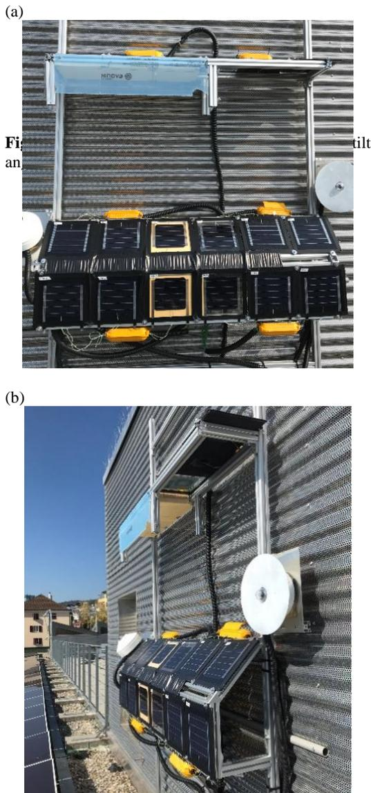
**Figure 2:** (a) Front and (b) side view of the mock-up structure used to monitor the temperature of the different samples. The mini-modules are facing south and are installed at three different tilts: 0°, 45°, and 90°. Two types of mounting configurations are used: full-insulation, and open-rack mount.
