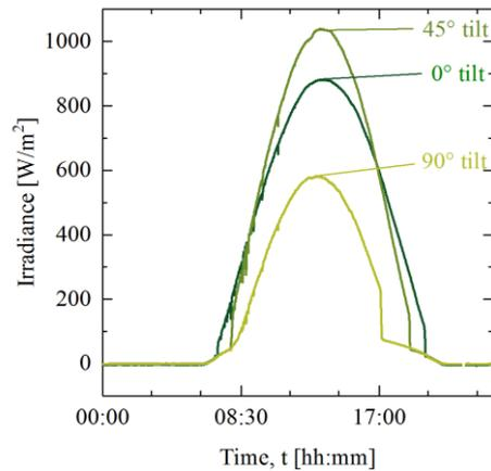
**Figure 4:** Irradiance measured for the different tilt angles at the end of summer (2018).
