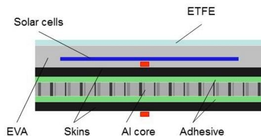
**Figure 1:** Schematic of a lightweight PV module structure. Each module is laminated with two thermocouples: one in direct contact to the solar cell and another placed at the back of the backsheet.
